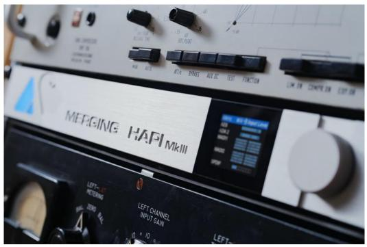
The Merging Hapi Mk III offers extensive routing capabilities for Dante and RAVENNA/AES67.
